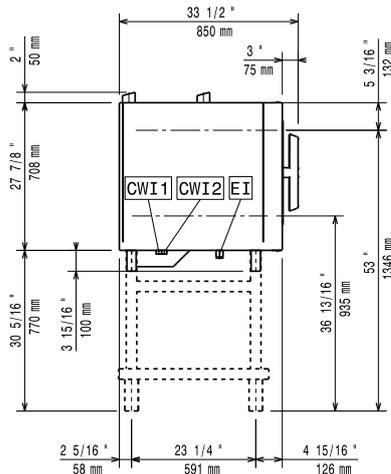
CWI1 = Cold Water inlet 1 (cleaning)      EI = Electrical inlet (power)
